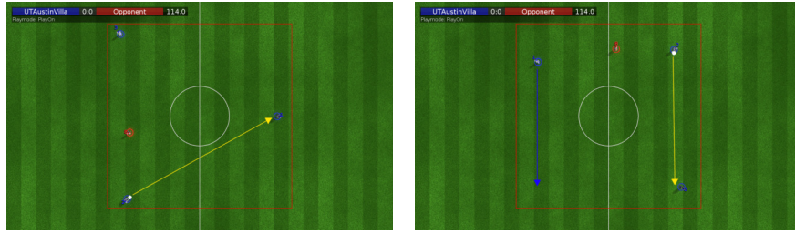
Fig. 3: Keepaway challenge triangle (left image) and square (right image) formations. Red box is keepaway area. Yellow lines show where ball will next be passed. Blue line shows agent movement using second level kick anticipation (moving to new position in formation once pass has occurred).
